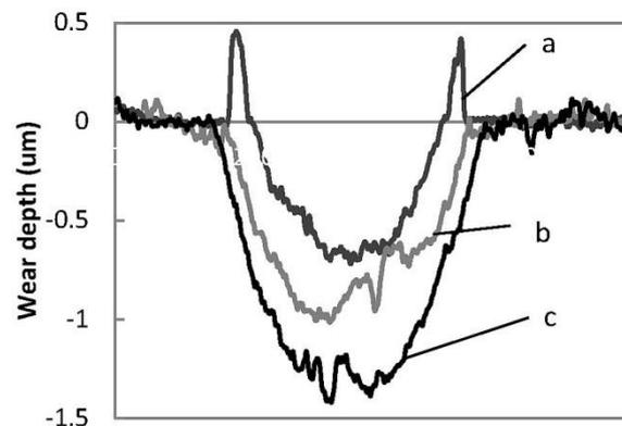
**Figure 4.** Depth profiles of wear tracks of Fe-W alloys (sample 1\_DC) after dry friction at 1 N (a), 2 N (b) and 5 N (c).
