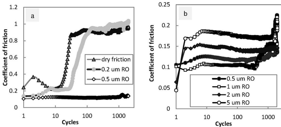
**Figure 8.** Evolution of the coefficient of friction at 2 N load applied on Fe-W sample 1\_DC in the presence of rapeseed oil (RO) film of 0-0.5  $\mu\text{m}$  (a) and 0.5-5.0  $\mu\text{m}$  (b) thickness. Lubricating conditions are indicated on the graph.
