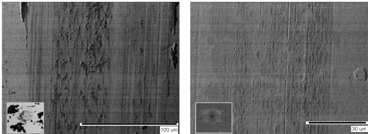
**Figure 7.** SEM images of the wear track after 2 N applied on Fe-25W sample after dry friction (a) and in the presence of 1 μm thick layer of rapeseed oil (b). In insert is the microscopic image of the corundum ball after the test.
