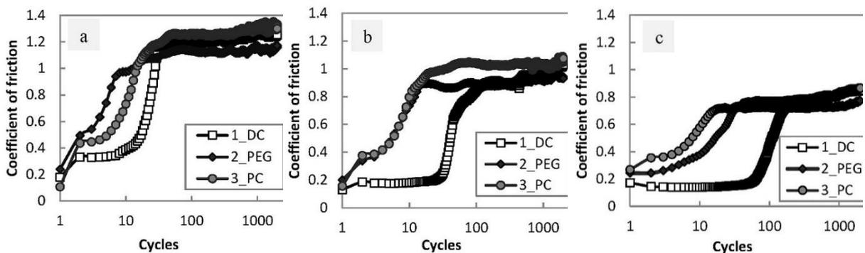
**Figure 3.** Evolution of COF of Fe-W samples at dry friction under applied loads: 1 N (a), 2 N (b), 5 N (c).
