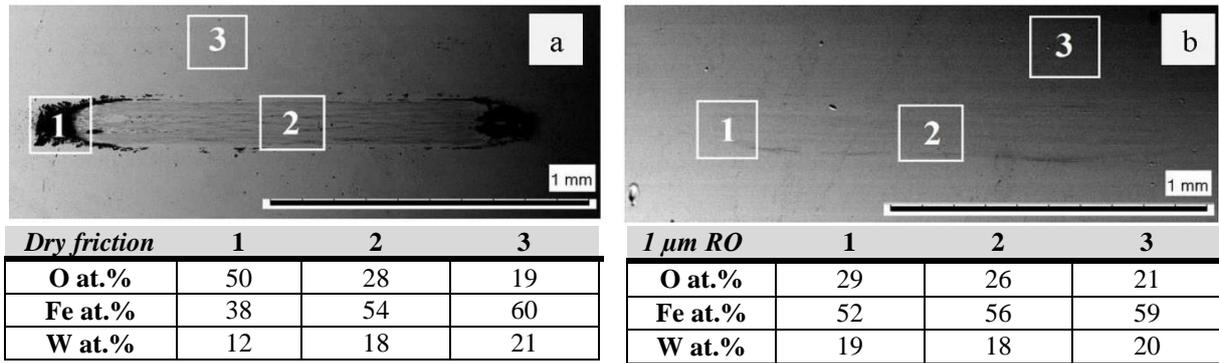
**Figure 6.** SEM images and EDS analysis of wear tracks on sample 1\_DC after fretting test at 2 N: dry friction (a); in the presence of 1 μm rapeseed oil (b); 1, 2 and 3 denote corresponding EDS analyzed zones.
