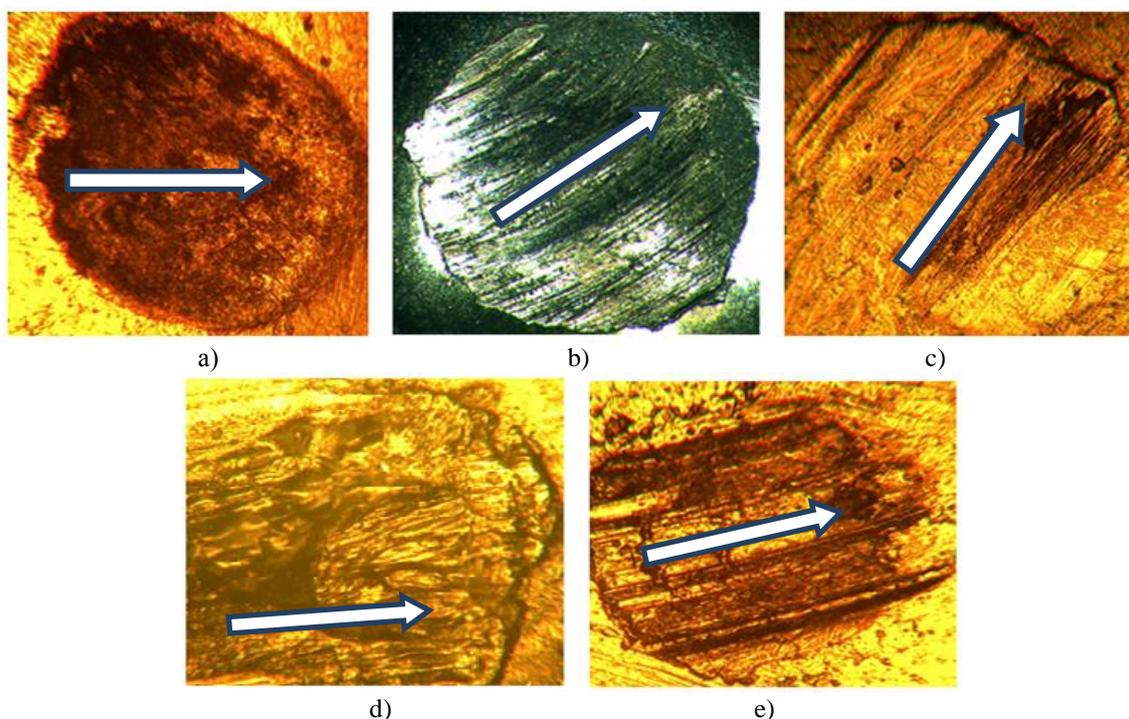
**Figure 9.** The wear spots of the balls at Pult for different lubricating oils, the arrow indicates the direction of motion. (The size of the wear spots is different; consequently the magnification range is different. It will not be correct to compare the microphotographs among themselves mechanically): a) without lubrication; b) beef fat; c) synthesized body of PET-acylglycerol 1/2, 35/65; d) lubricant based on PET-acyl glycerol 1/2, 35/65; e) Lithol-24.
