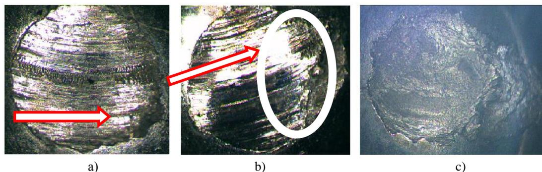
**Figure 10.** Spot wear of the ball with  $P_{weld}$  for different lubricating oils: a) beef fat; b) synthesized body of PET-acylglycerol 1/2, 25/75 (the circle highlights the area of brittle failure); c) Lithol–24.
