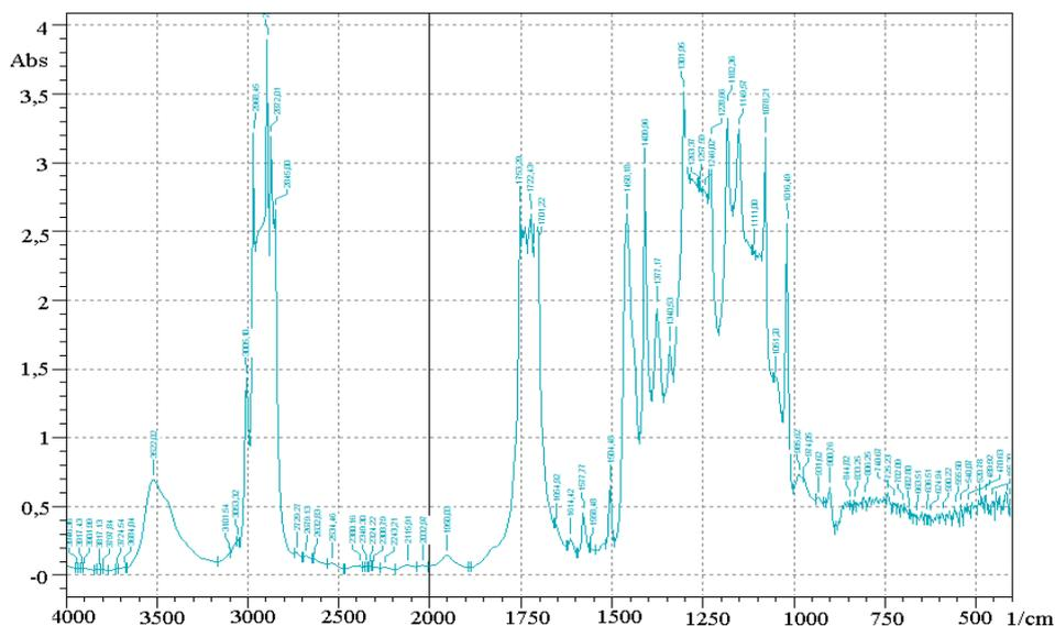
Figure 4. IR spectrogram of PET-acylglycerol based on rapeseed oil.
