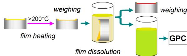
**Figure 2.** Procedure of “PennState microoxidation” test by heating the film, weighing volatile losses, dissolving the degraded film in solvents and analyzing the soluble portion with Gel Permeation Chromatography.
