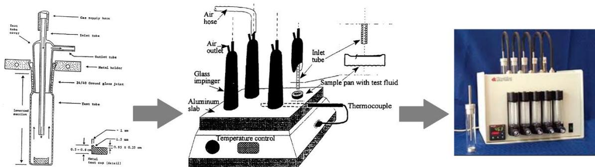
**Figure 3.** Historical transformation of PennState micro-oxidation test (left, reported in [5]) into a version without a liquid metal bath (center, reported in [6]) and a commercial version K29200 (right, reported in [7]).
