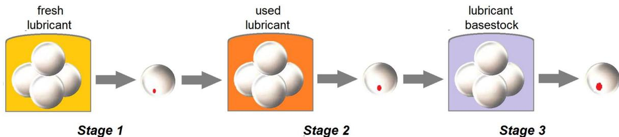
**Figure 1.** Procedure of sequential 4-ball wear test, using three stages with intermediate wear scar measurements. Synergistic additives should result in little wear scar increase after stages 2 and 3.
