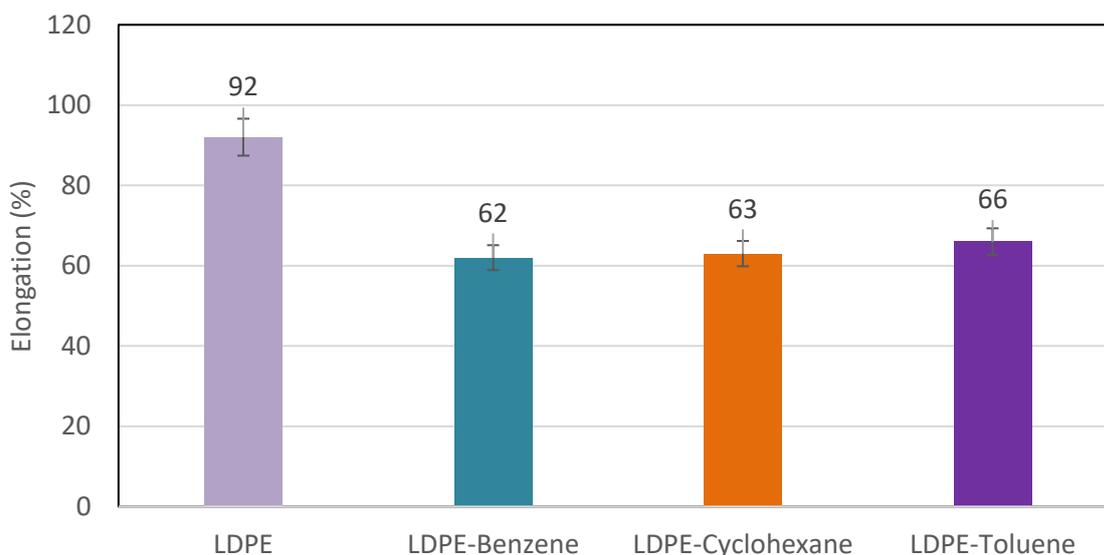
**Figure 2.** Tensile elongation at break for dry LDPE (left) and for LDPE subjected to swelling in several solvents.
