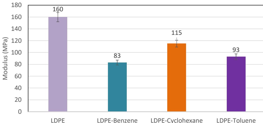
**Figure 1.** Tensile modulus values for dry LDPE (left) and for LDPE subjected to swelling in several liquids.
