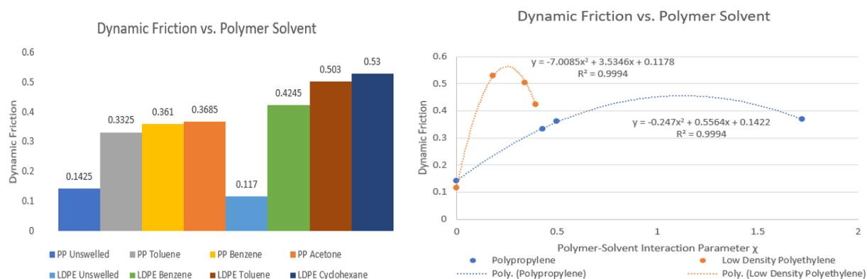
**Figure 3.** Dynamic friction values as a function of the polymer-solvent interaction parameter  $\chi$ .
