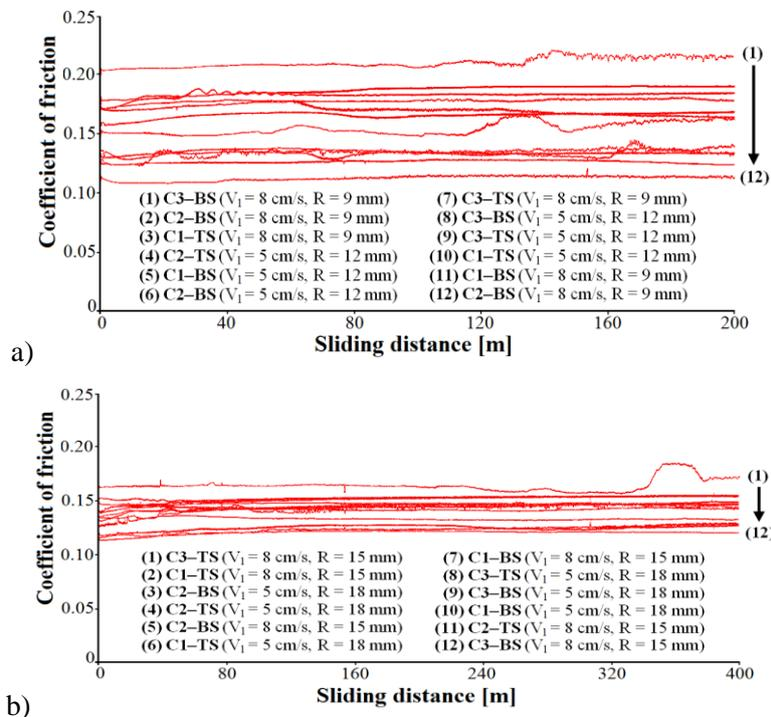
**Figure 2.** Variation of CoF with sliding distance: (a) L = 200 m, (b) L = 400 m, for W-Cu composites.
