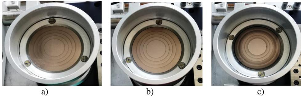
**Figure 1.** Aspect of TS surfaces of W-Cu composites: (a) C1, (b) C2, and (c) C3, after ball-on-disk tests in oil.
