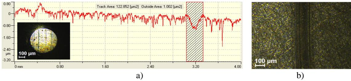
**Figure 3.** Wear track profile recorded for C1–TS surface ( $P = 30\text{ N}$ ,  $V_1 = 5\text{ cm/s}$ ,  $R = 12\text{ mm}$ ,  $L = 200\text{ m}$ ) (a), along with optical images of worn track width (b) and diameter of the removed cap from the ball (inset of (a)).
